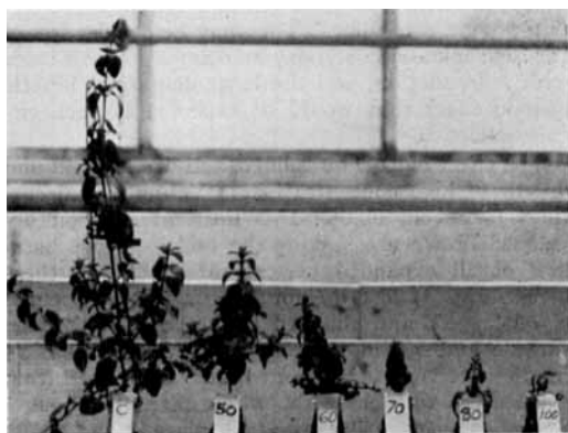
Fig. 3.—Peppermint plants grown in liquid nutrient solutions containing 50 to 100% D_2O .
